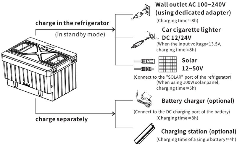
**Note:** It is suggested to switch off the refrigerator when charging the battery (the power supply may mainly power the compressor when the refrigerator is running).
